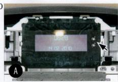
If the two button display is installed there is no trim required
