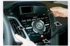
Remove the OEM panel using a plastic wig
