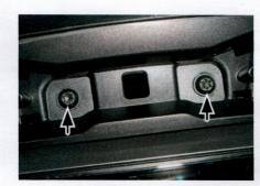
Remove the scews using a Torx T25
