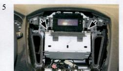
Remove the original headunit using a Torx T25
