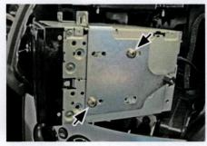
Place the mounting brackets on the new headunit and place the headunit
