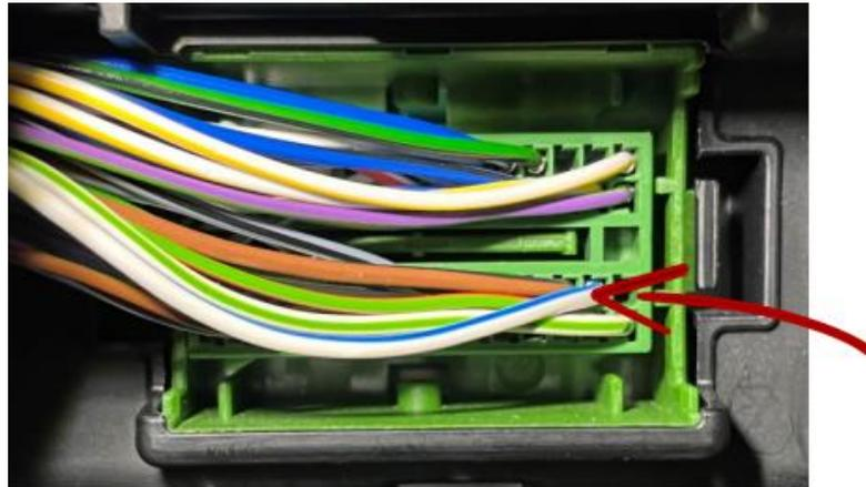
The REVERSE SIGNAL is located in the green connector, Pin 17, blue-white cable.
