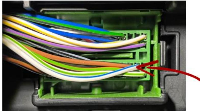
The REVERSE SIGNAL is located in the green connector, Pin 17, blue-white cable.
