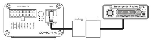
The CO-40.4 M offers MAIN input, which is connected by High or Low Level to the output of the head unit and an AUX input, which is connected by a 3.5mm jack to an AUX source. If the amplifier detects a signal at AUX it will automatically turn on. Priority 1 is always the AUX input. If there is any signal detected at AUX the amplifier will play the AUX source through the outputs.
