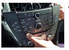
6. Unclip and remove OEM head unit
