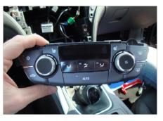
Remove air condition control unit from OEM panel
