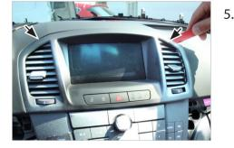
Unclip and remove OEM display
