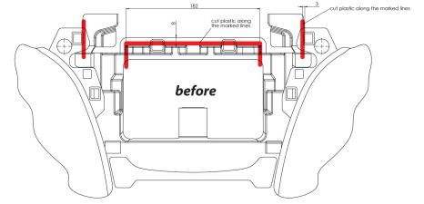
10. Cut plastic from dash board in order to clear space for the double DIN head unit (see lines in the drawing)
