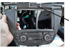
11. Mount air condition control unit to double DIN facia place
