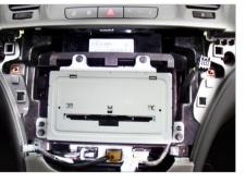
7. Remove OEM cd/radio parts
