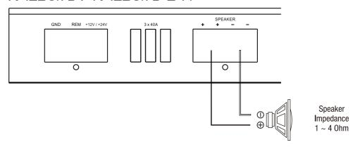
Please note that this unit is a mono block amplifier and has only one channel. Connecting to either the positive or negative of either of the two connections will end in the same result as both positive connections (or both negative connections) are tied together inside the unit. For example, if you connect two 2 ohm subwoofers, the amp will parallel the connections for a 1 ohm load.
