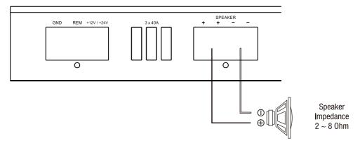
Please note that this unit is a mono block amplifier and has only one channel. Connecting to either the positive or negative of either of the two connections will end in the same result as both positive connections (or both negative connections) are tied together inside the unit. For example, if you connect two 4 ohm subwoofers, the amp will parallel the connections for a 2 ohm load.
