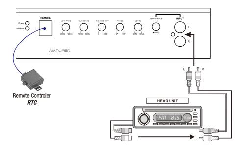
The SERIES amplifier offers RCA-Inputs, which are connected through cinch cables with the preamplifier-outputs of the head unit. IHLAC and RCA IHI adapter cable can be purchased as accessories if the head unit has no RCA output. The HI/LOW button must be switched to "HI". If the SERIES amplifier gets a signal from head unit output, the amplifier will turn on.
