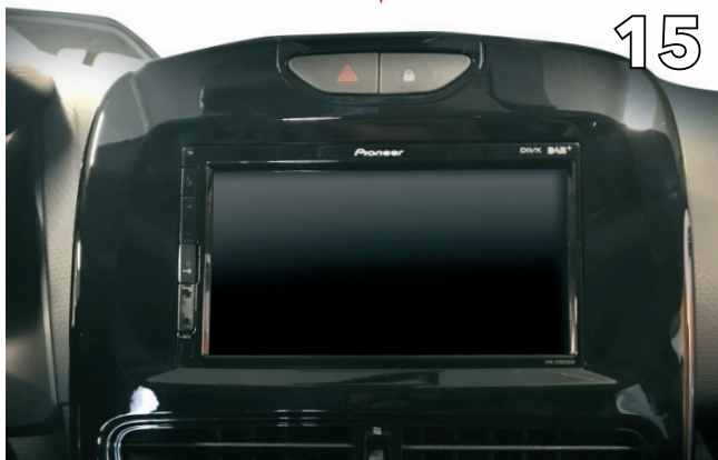
Put the fascia into the car and click the correct hazard switch cover in position
