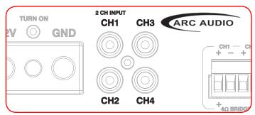
In this case it is recommended that you use an appropriate RCA cable with one set of ends removed as inputs for the amplifier.
